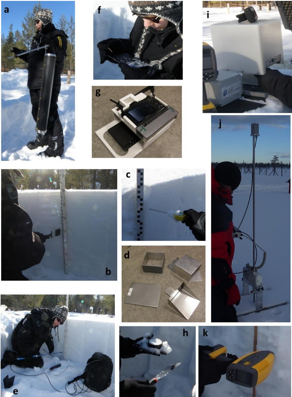
Figure 7. Photos of snow pit instrumentation: a) bulk SWE with Korhonen-Melander sampler, b) stratigraphy, c) temperature, d) 500 cm 3 and 250 cm 3 density cutters, e) SnowFork, f) visual estimation of snow grains, g) camera and stand for macro-photography, h) IceCube sampling, i) IceCube, j) SMP, and k) QST. Modified from Publication V.
