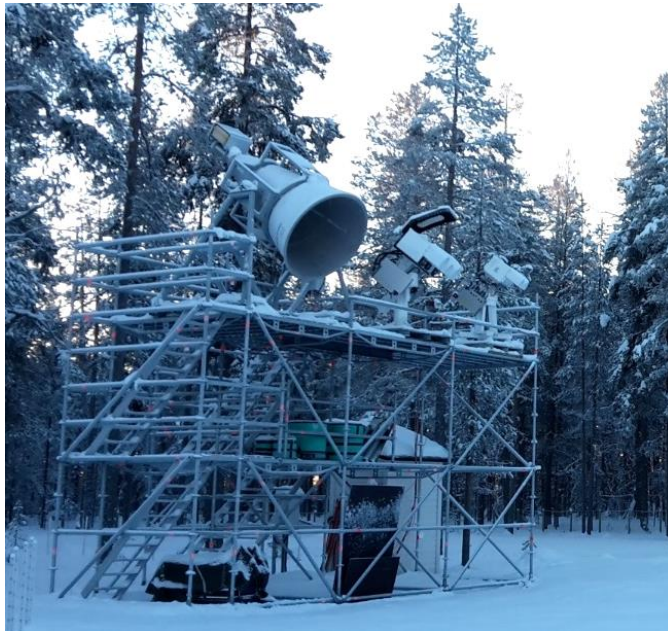
Figure 8. Tower-based ESA ELBARA II (left), SodRad1 (middle), and SodRad2 (right) radiometers at IOA.
