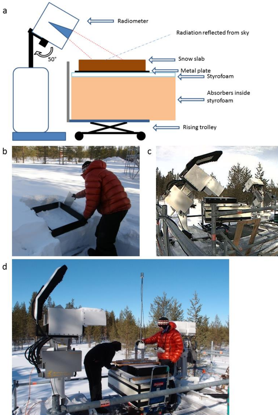
Figure 9. a) ASMEEx setup. Reprinted from Publication IV. b) Excavation of snow slab for ASMEEx. Modified from Publication IV. c) Radiometric measurement of the slab with SodRad1 radiometer. d) SMP measurement from the snow slab.
