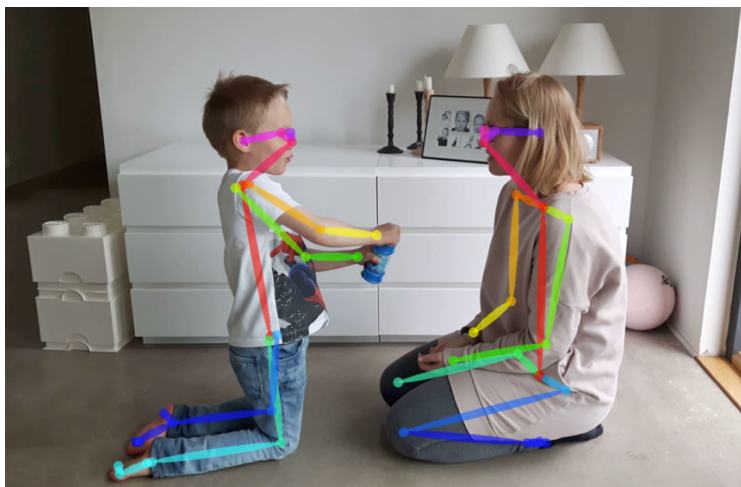
Figure 2. A video frame with body key points detected with the OpenPose (Cao et al., 2018). Subjects have given permission to use the picture.
