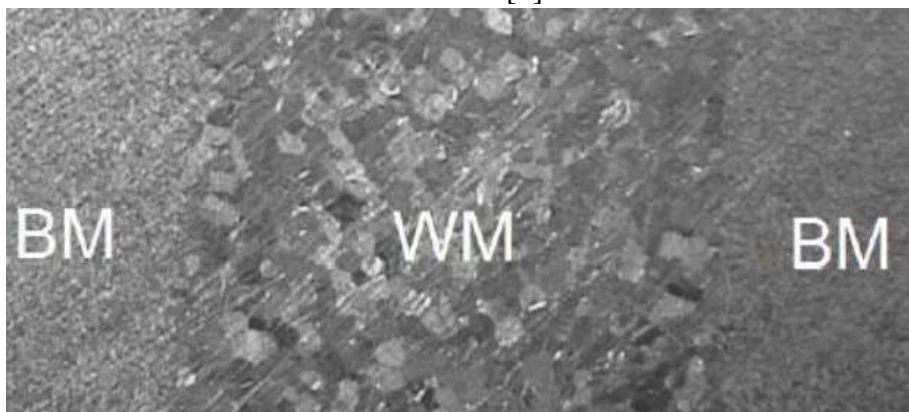
Figure 1: Macrostructure of the welded joint [1]
