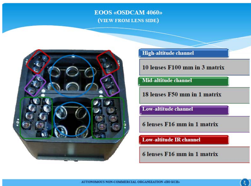
Figure 3: The Russian Open Skies camera system OSDCAM 4060 (source: www.poksi.ru/OSDCAM_44060-Eng.pdf , access 12. August 2019)
