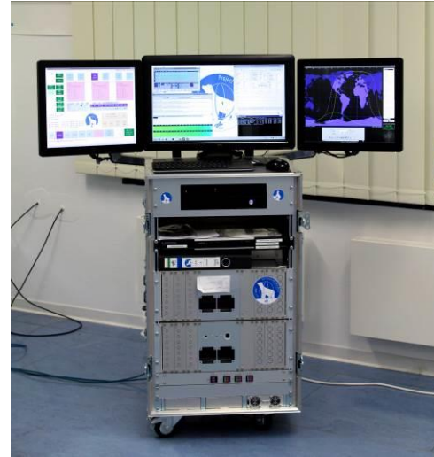
Fig 3. Remote controlled user terminal with application software
