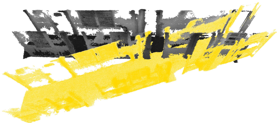
Figure 1.6: Two not registered point clouds capturing one scene, differing by a rotation.
