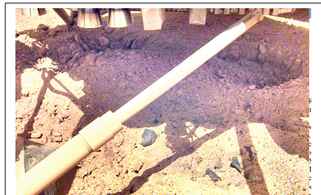
Fig. 4. Image under the lander showing struts, retrorockets, excavated pits (~10 cm deep), dark gray aphanitic rocks (basalt) and duricrust. Note steep pit walls of soil and clasts indicating cemented duricrust and clods and fragments that litter the pits and surface.
