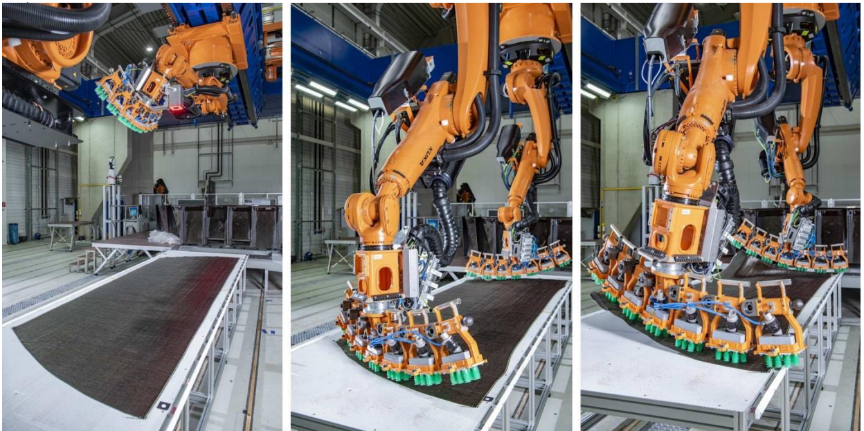
Fig. 6: Future factory layup: Detection, start of gripping, end of gripping
