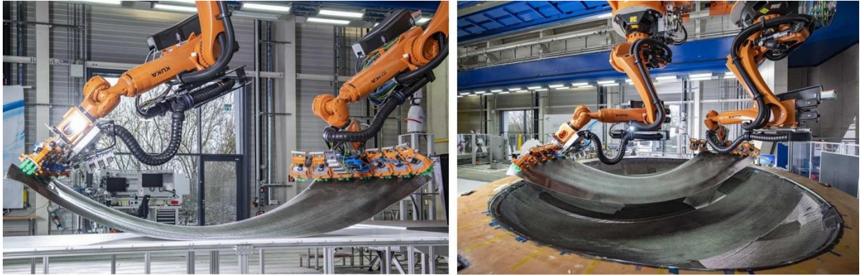
Fig. 7: Future factory layout: Cut piece lifted, transferred and ready to drop.
