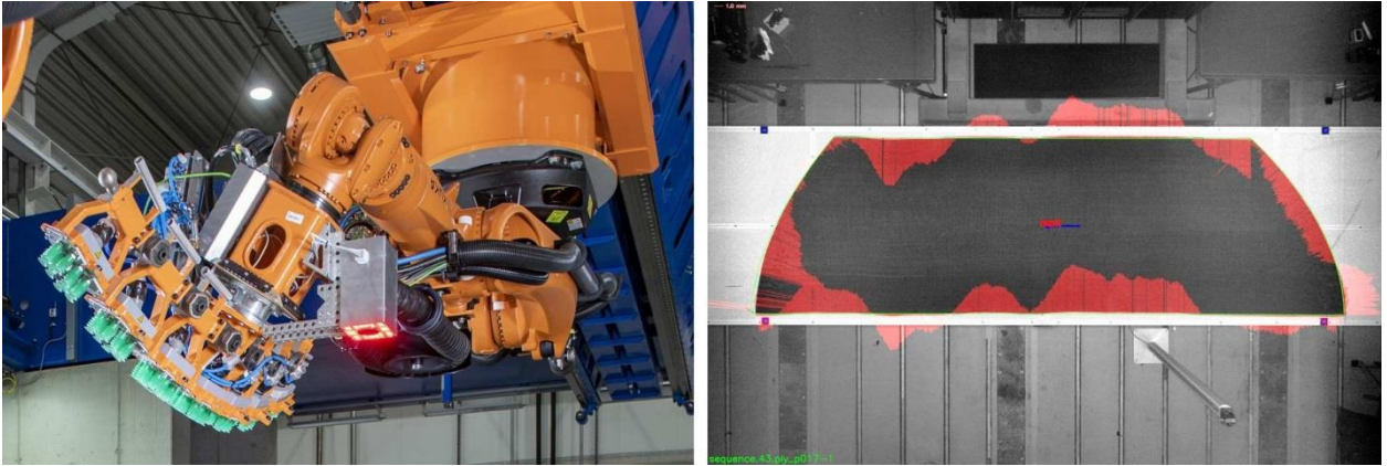
Fig. 2: Camera for cut piece detection mounted to one of the robots with detection result. The deviations from the ideal shape are drawn in enlarged form.
