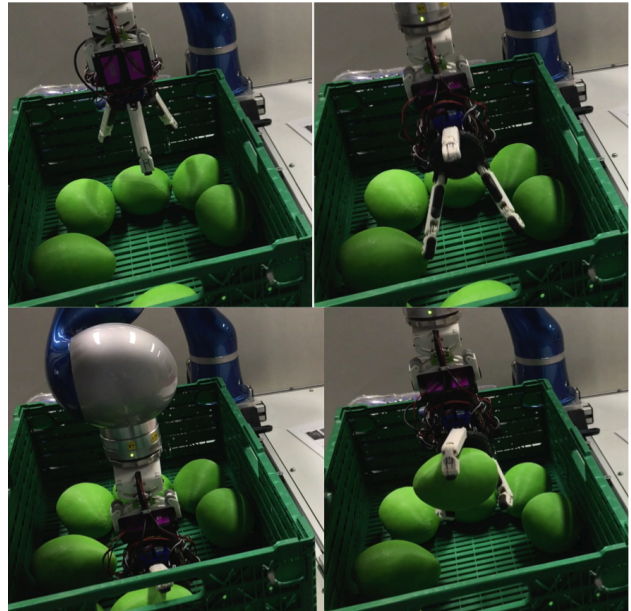
Fig. 6: wall grasp sequence of a mango
