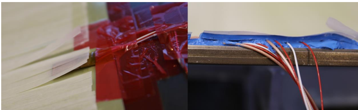
Figure 5 - Sensor integration during production
