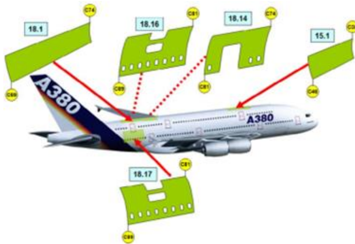
Figure 1: GLARE fuselage panels made by Tier-1-Supplier PAG in Nordenham /Germany [4]
