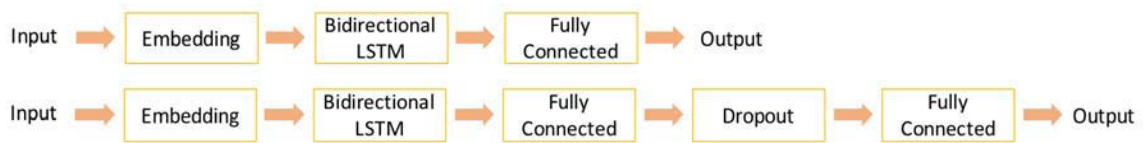
Figure 3.4: Architectures of model m1 (top) and model m2 (bottom)
