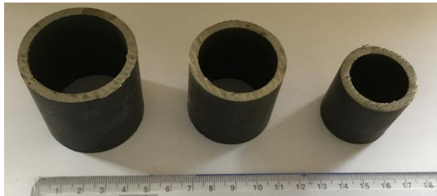
Figure 3. Hollow steel sections (caps)
