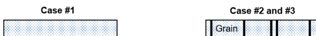
FIG. 6. Illustration of 1D nanocomposites. The average grain size is 1.3 \mu\text{m} , and the material properties of the grains and grain boundaries are the same as for the 2D samples considered in Fig. 5. Case 1: Uniform material. Case 2: Nanocomposite with reduced \kappa in grain boundaries. Case 3: Nanocomposite with reduced \kappa and enhanced S in grain boundaries.
