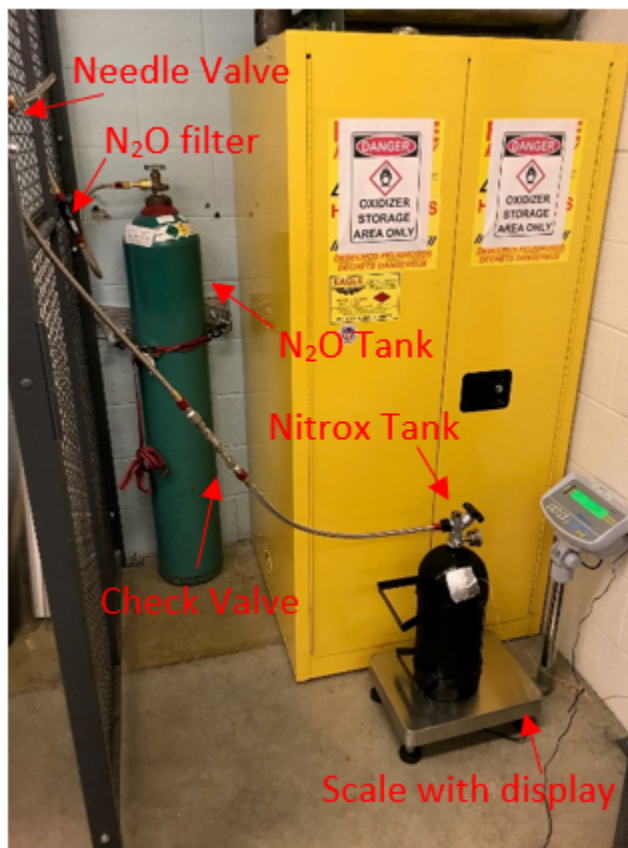
Fig. 2.6: N_2O Fill Apparatus [3]
