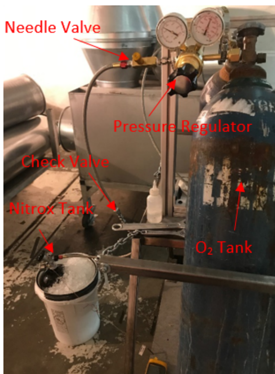
Fig. 2.7: Assembled O_2 Percolation Apparatus [3]
