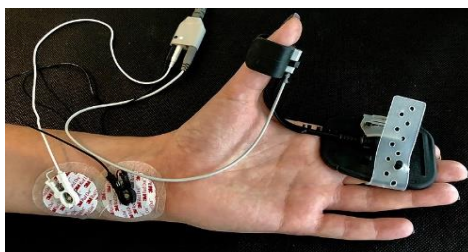
Figure 1.1: Surface EMG sensor. Picture by Paul Anthony Stewart published under Creative Commons Attribution-Share Alike 4.0 International license on Wikipedia Commons
