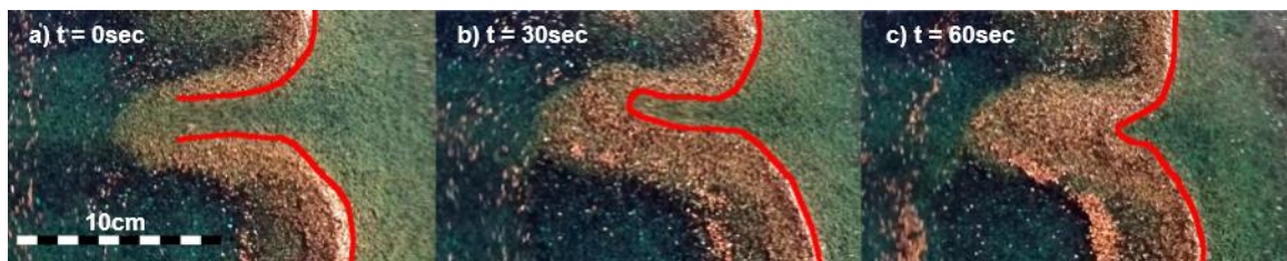
Figure 13: Progression of an overwash channel to a ridge. All three photos are taken at the time of maximum swash of a wave. a) An open overwash channel that is approaching the maximum length that the waves can transport sediment across. b) The same overwash channel once sediment was deposited in the outlet, blocking future waves. c) The former overwash channel after the majority of it has been filled in.
