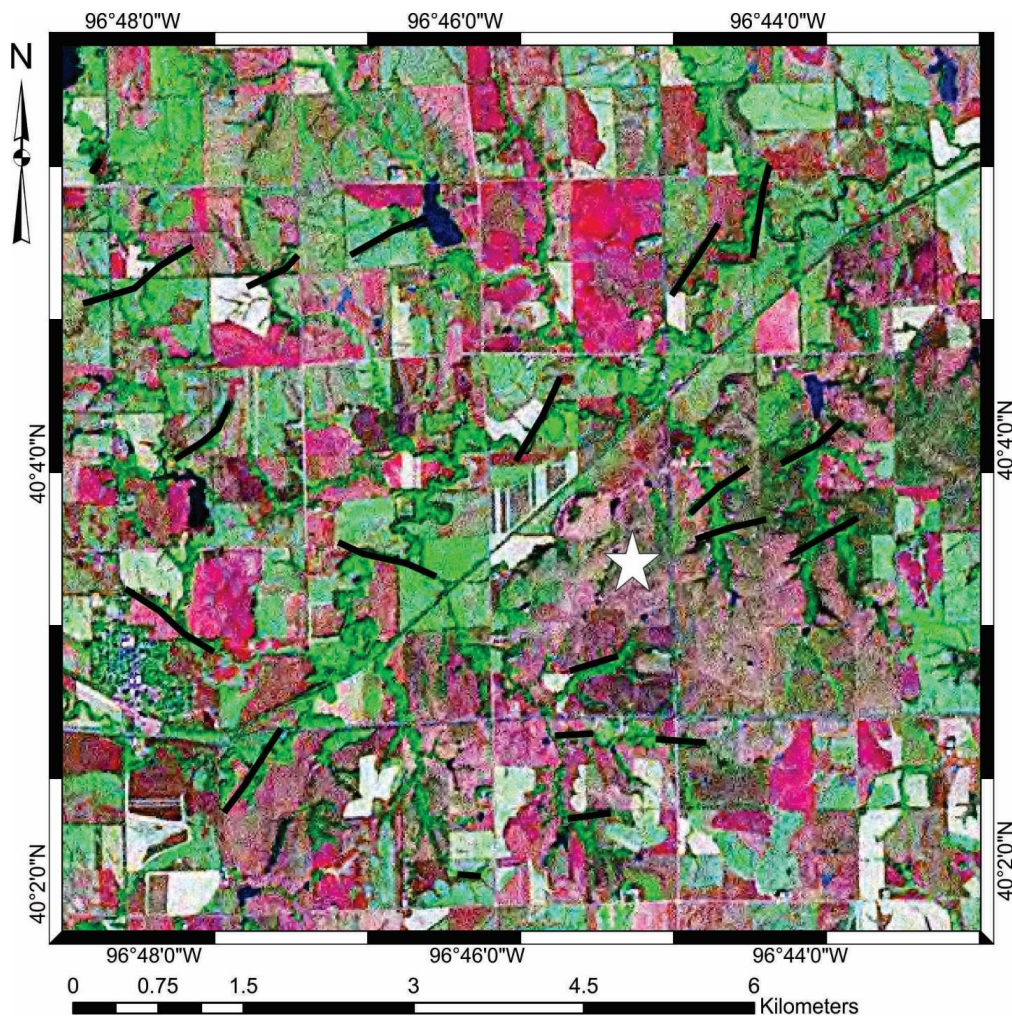
Figure 7. MrSID image from Figure 4, above, this time with lineaments marked in black. White star represents the location of site NF 3.
