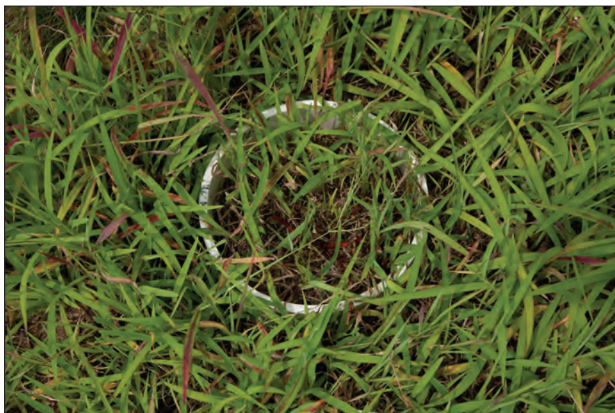
Figure 6 Natural-shallow ring installation. Vegetation was left undisturbed if it did not interfere with the proper seating and function of the accumulation chamber.
