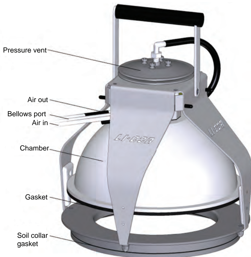
Figure 3 Detail of the soil CO 2 flux monitoring accumulation chamber. From LI-COR Inc. (2015). Used with permission.
