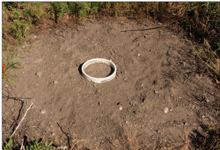
Figure 5 Bare-shallow ring installation with vegetation removed (approximately 0.5-m [1.6-ft] radius from the center of the ring).
