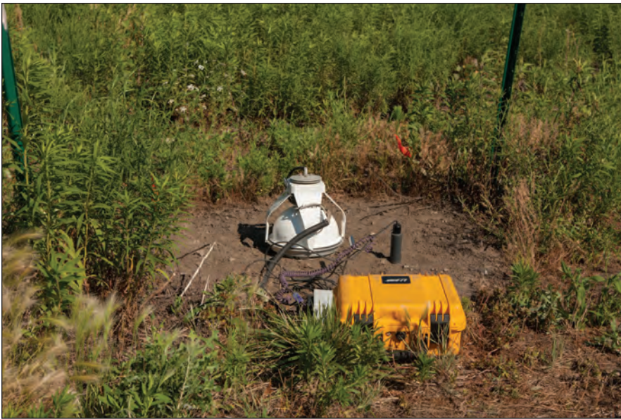
Figure 4 LI-8100A analyzer control unit and accumulation chamber during field use at a bare-shallow installation.
