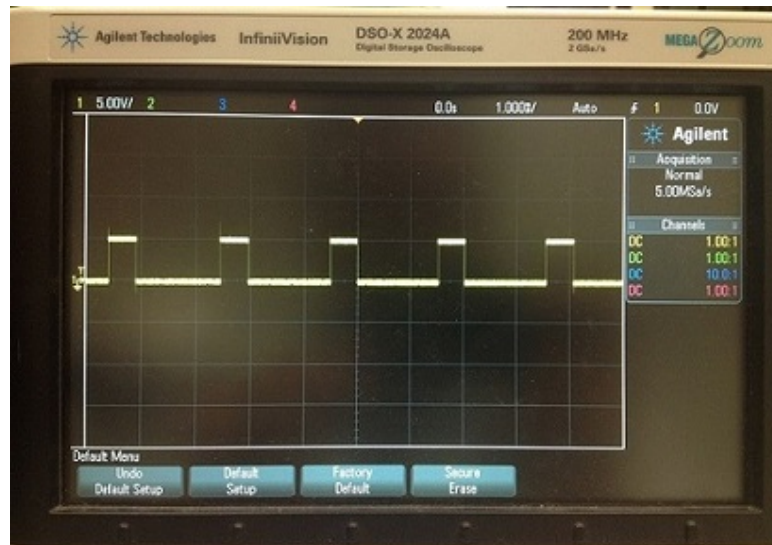
Figure 4.5: Output PWM signal (5v) from CPU.
