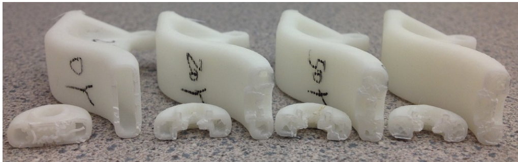
Figure 5.6: The fracture surface of parts made along the Y axis. From left to right, the filling percentages of the body are 0, 20%, 50%, and 80%.
