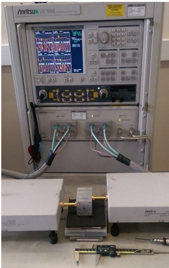
Fig. 4 Measurement setup of the higher order mode coupler.
