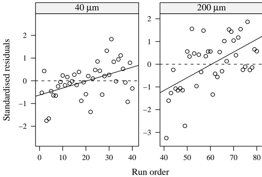
Figure 2: Standardised realisations of the residuals of the model in equation 2 versus the sequence of the tests.
