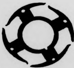
Figure 3.22 A skewed-pole lamination
