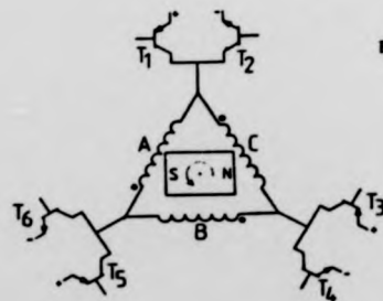
d) Commutator replaced by electronic switches
