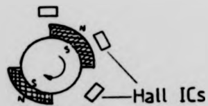
Figure 3.27 An arrangement of trigger magnets and Hall-effect ICs
