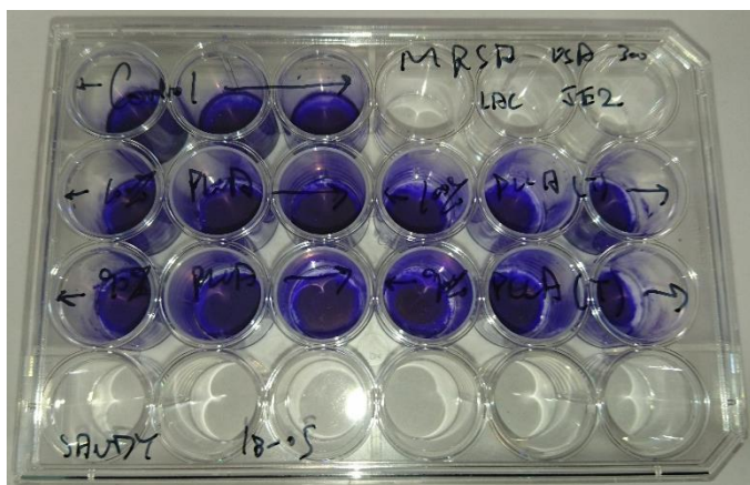
Figure 4.19. Photograph of a multi-well plate with stained biofilm on the composite materials.
