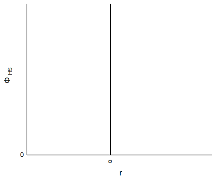
Figure 2.8: The potential energy as a function of distance for the hard sphere potential.
