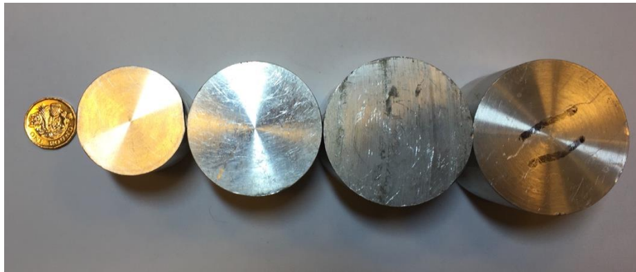
Figure 3.1: Full range of diameters for cylindrical deployment objects for the large-scale apparatus, including the smallest 4.2 cm diameter sample to the left, to the largest 6.0 cm diameter sample to the right. £1 coin added for comparing scale.
