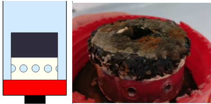
Figure 3.5: Damping and draining mechanism used in the wide bore apparatus (see main text for details: a) schematic, b) actual photograph.
