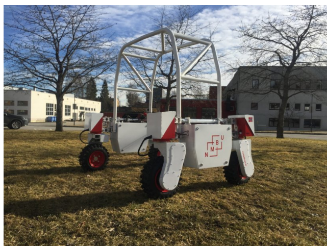
Fig. 5. The Thorvald II robot specifically designed for phenotyping tasks, with narrower wheels, higher ground clearance, and a modular design allowing us to rebuild the robot into a wide variety of configurations and sizes.
