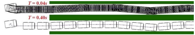
Fig. 16. Simulation: strobe pictures of robot tracking a defined trajectory with different strobe periods T . The utilized parameters for control and reference were [5]: v_{rx} = 0.35 \text{ m/s} (in linear tracking), \omega_r = 0.5^\circ/\text{s} (in rotations), a = b = 29 \text{ mm} , c = 25.5 \text{ mm} , r = 20 \text{ mm} (wheel radius), x_{irc} = 0 \text{ mm} , \alpha_0 = 1 , \alpha_1 = 0.5 , \epsilon_1 = 0.01 , k_1 = k_2 = 50 , z_{d1}(0) = z_{d2}(0) = 0.45 .
