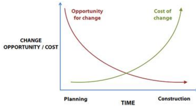
Figure 3: Change vs. Cost of Early Project Decisions adapted from Cambridge Institute for Sustainability Leadership (2015)
