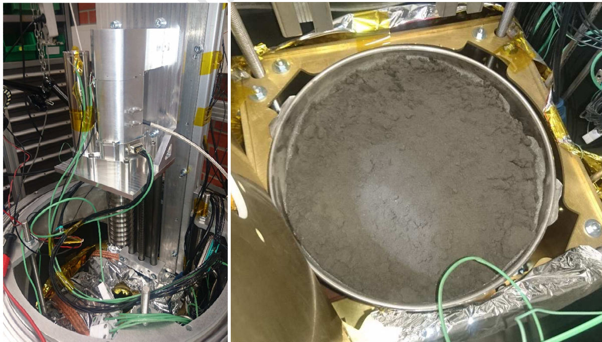
301 Figure 9: Left: Image of the LVS on the vertical actuator inside the thermal vacuum test setup. Right: Image of a hydrated 302 frozen JSC-1A sample in the sample container.
