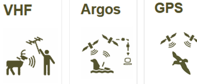
Figure 2.3: Graphic representation of the three main technologies used for tracking animals. VHF tags convey radio signals picked up with an antenna; position is obtained through triangulation. ARGOS devices send Doppler Shift signals to the satellites which transmit the signal back to a user computer. GPS loggers receive signals from the satellites and store them into their internal memory; loggers need to be retrieved in order to download the data into a computer (© 2016 www.sirtrack.co.nz ).
