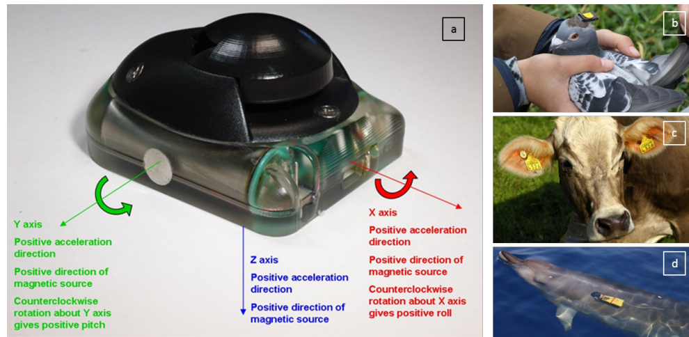
Figure 2.4: A sampling of bio-sensors: a) external design and description of the direction axes of a Daily Diary (DD) logger (© www.wildlifecomputers.com ); b) neurologger partially implanted in a homing pigeon's skull for studying spatial cognition of the species (Vyssotsky et al., 2006); c) UHF RFID proximity tags attached through perforation on cattle ears for identifying them (© www.rfidreaderuhf.com ); d) Time-Depth Recorder (TDR) logger attached on the back of a beaked whale by means of a suction-cup (© www.savethewhales.org ).
