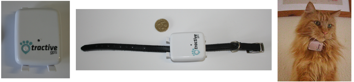
Figure 5.2: The Tractive device. On the left, the white case; on the centre, the collar attached to the case with an old UK pound coin for scale (coin: 23mm diameter); on the right, the device worn by a cat participant.
