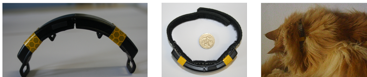
Figure 5.1: The PawTrax device. On the left, the two black cases hinged together and completely bent; on the centre, the collar attached to the case with an old UK pound coin for scale (coin: 23mm diameter); on the right, the device worn by a cat participant.
