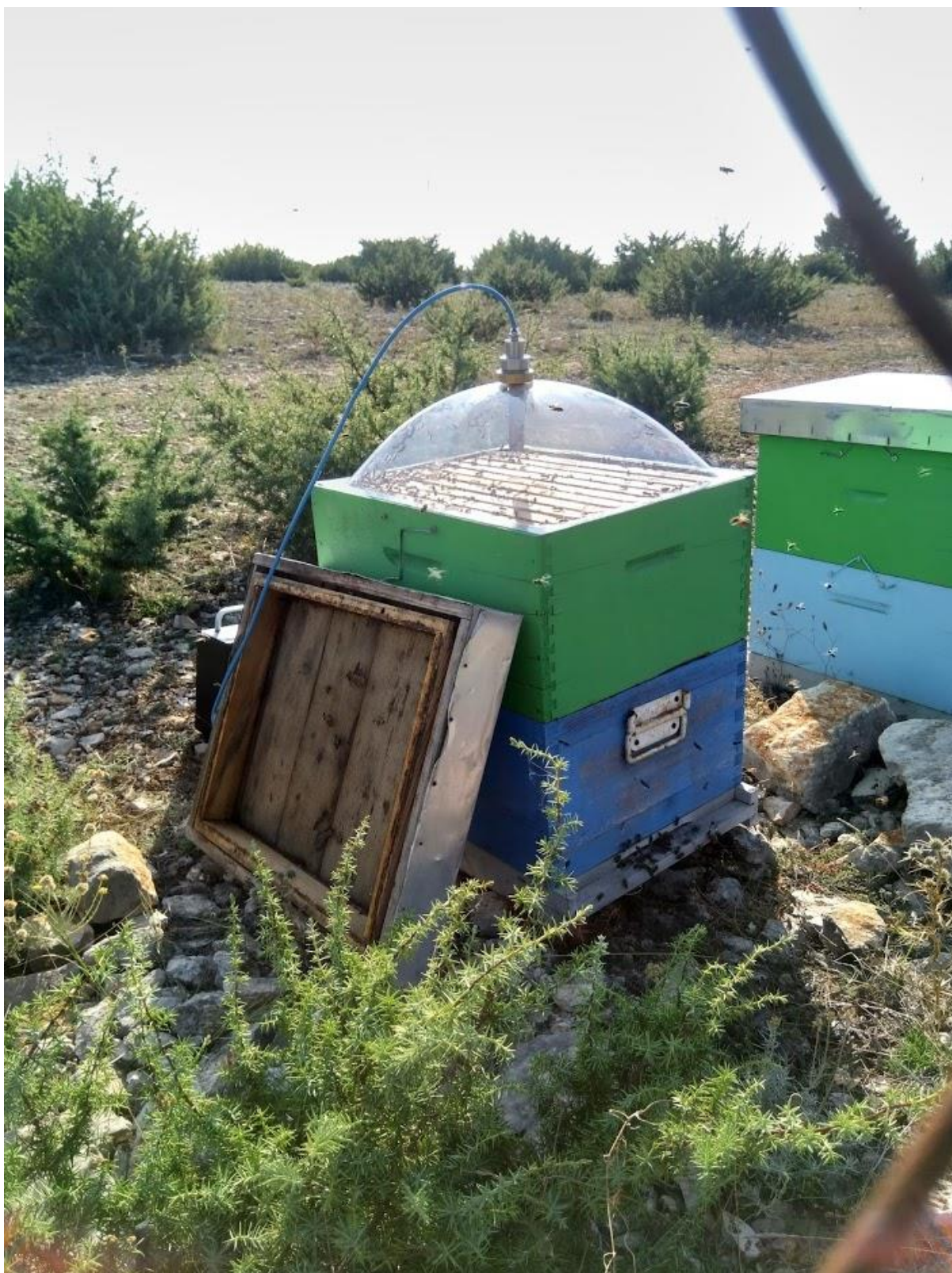
Figure 8 – Air sampling via specialised cupola on top of the bee hive.
