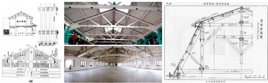
Fig.2. Chinese traditional carpentry and Modern Chinese roof trusses under Western influence.
