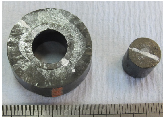
Figure 1. A photograph of the single grain GdBCO ring-shaped sample and a 12 mm diameter single grain cylindrical (core) sample.
