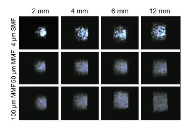
Figure 62 Near-field images of the waveguide output for different bending radii under different inputs. Bending radii were chosen to be 2 mm, 4 mm, 6 mm and 12 mm.
