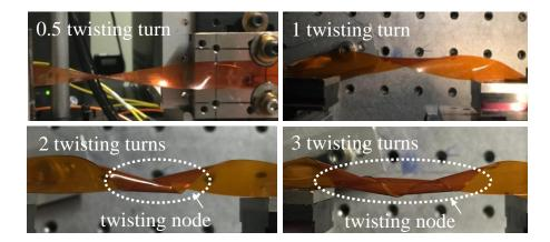
Figure 69 Twisting patterns of a flexible polymer waveguide sample for different numbers of twisting turns. When twisting turn is bigger than 1, twisting nodes are generated. Waveguide sample is 10-cm long and 1-cm wide.
