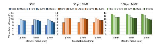
Figure 101 5% FFAs of the emitted beam at the waveguide output under different bending radii and turns and different input launch conditions.
