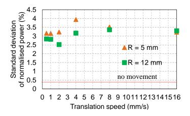
Figure 87 Obtained standard deviation values as a percentage of the mean value of the received power for different bending
