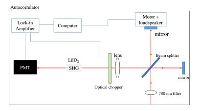
Figure 123 Diagram of the home-made autocorrelator used in this work.
