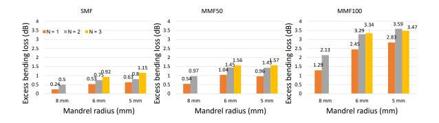
Figure 100 Excess bending losses of a flexible polymer waveguide for the small bending effect under three different input conditions. Mandrel radius is set to be 5 mm, 6mm and 8 mm. Bending turns is chosen from 1 to 3.
