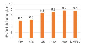
Figure 129 5% FFAs of different input excitations for ultra-short laser pulse measurements. Input launch conditions are chosen from most restricted one: ×10 lens to relatively restricted one: 50 µm MMF. All launches are under-filled.
