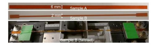
Figure 71 Flexible polymer waveguide samples used in twisting loss measurements: (a) sample A 24 cm long with 6 mm width and (b) sample B 24 cm long with 2 mm width, and (c) image of twisted sample B under 5 full (360°) twist turns.
