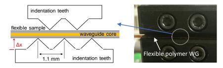
Figure 103 Schematic diagram of mode scrambler and an image of the system setup for micro-bend measurement. Force is applied on the waveguide due to the squeeze of teeth, generating micro-bends.
