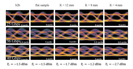
Figure 138 Received eye diagrams at different transmission speeds for the b2b and waveguide links for the different radii applied to the 1 m spiral waveguide sample.
