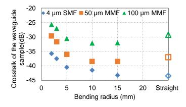
Figure 80 Crosstalk performance of the flexible waveguide sample when bending at different radii under different launch conditions. Results when waveguide sample was in straight condition are also indicated by unfilled markers.
