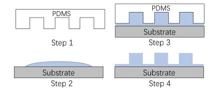
Figure 13 Soft lithography method for fabricating polymer waveguides. A mould is needed to be built first which is made of PDMS material. A remnant layer can be generated as the core material cannot be fully expelled by the mould, which results
