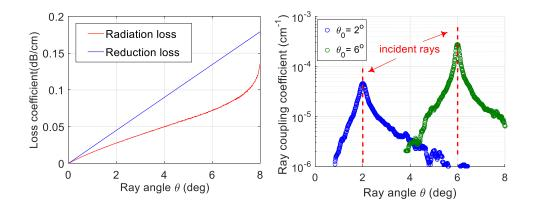
Figure 111 Radiation and reduction loss coefficients as a function of propagation angle  $\theta$  due to the surface roughness and ray coupling coefficients for the reflection of a single incident ray of unit power at two different  $\theta$  angles [150].
