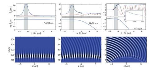
Figure 34  $TE_0$  bent mode profiles and snapshots of propagating bending modes. Waveguide structure is set to be bent at 200  $\mu$ m, 50  $\mu$ m and 10  $\mu$ m from left to right, respectively [123].
