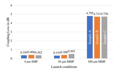
Figure 56 Coupling losses for different waveguide samples under three input launch conditions.
