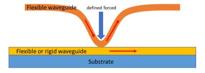
Figure 21 Schematic of bent waveguide coupling scheme. A curved waveguide is generated due to the defined force. Some optical power therefore will leak out of waveguide in this curved waveguide region. Partial leakage power will re-couple back to the straight waveguide. The coupling efficient for this method is currently around 35%.
