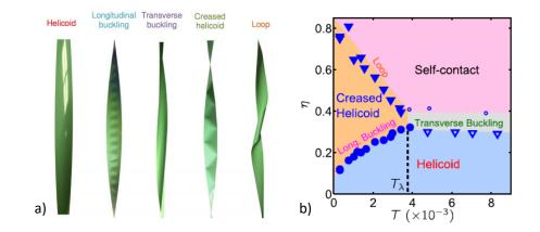
Figure 73 a) Buckling modes of twisted ribbon, there are five patterns: helicoid, longitudinal buckling, transverse buckling, creased helicoid and loop, b) experimental phase diagram in the tension-twist plane [137]
