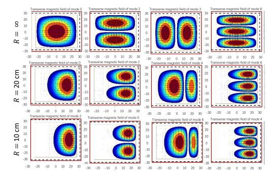
Figure 35 Example of some bending modes in multimode waveguides at different bending curvatures, R = 10 cm and R = 20 cm. Waveguide modes in straight waveguide  $R = \infty$  are given for comparison as well.
