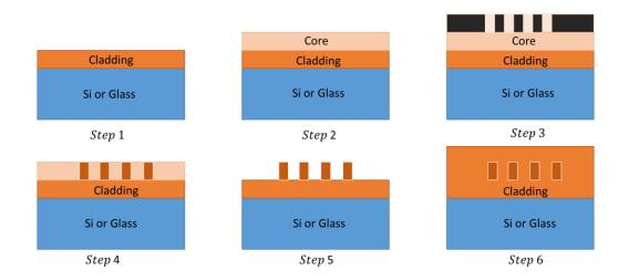
Figure 12 Common polymer waveguide fabrication steps based on photo-lithography method. Waveguide core material is photo-sensitive, and a variety of materials can be chosen as substrate depending on different purposes.
