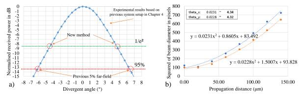
Figure 120 a): Blue dotted line is the far-field power distribution of the SMF output. 5% FFAs are the angle values when its far-field profile intersects with red dash line (-13 dB). Green dash line indicates the new far-field angle results obtained from using ISO-11146 method. b): curve fitting of un-focused beam width. New far-field angle is calculated as square root of
