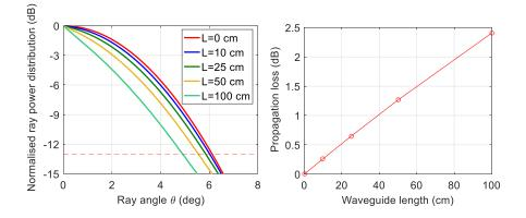
Figure 113 Simulated ray power distribution and propagation loss for different waveguide lengths for a Gaussian ray input power distribution with a 2.5° standard deviation [150].
