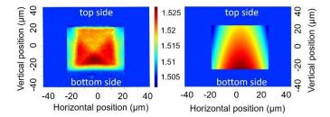
Figure 60 Measured refractive index of the waveguide sample and simulated profile in ZEMAX for flexible waveguide studies. The simulated profile has roughly the same RI distribution as the real waveguide sample.
