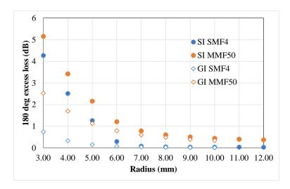
Figure 39 Simulated bending loss performance of step-index (SI) and graded-index (GI) waveguides under different launch conditions. Filled are SI waveguide simulation results and unfilled are GI waveguide simulation results. Bending degree is set to be 180° in both cases.
