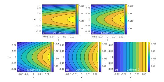
Figure 43 Different refractive index profiles of waveguide core, with parabolic shape changes in y-direction.
