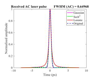
Figure 126 AC laser pulse under the 50 µm MMF input fitted by Gaussian, Sech<sup>2</sup> and Lorentzian curves. FWHM of AC pulse is measured to be 0.64968 ps.
