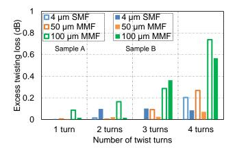
Figure 72 Average twisting excess loss for samples A and B as a function of the number of full 360° twists for the different launch conditions. Unfilled bars are the results of sample A and filled bars are the results of sample B.
