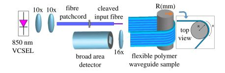
Figure 58 Experimental system setup for bending loss studies. An 850 VCSEL is used as the input source. Laser light is coupled into fibre patch-cord first and next coupled into the bent waveguide. The waveguide sample was bent at 180°. At the receiver side, a broad-area PD is used to collect the power via a ×16 lens.
