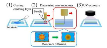
Figure 15 Mosquito method for fabricating circular graded index profile of polymer waveguides. Waveguide core material is injected into cladding via a needle along propagation direction and waveguide core size is controlled by the scanning speed. After core monomer diffusion, a graded index profile can be formed [92].
