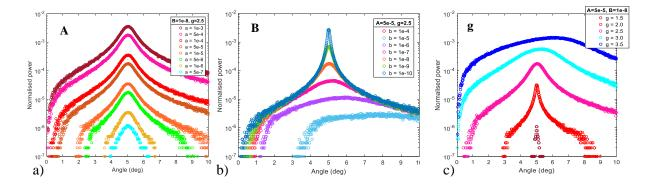
Figure 110 Scattered ray responses due to the change of ABg parameters, a) change of parameter A, b) change of parameter B and c) change of parameter g.
