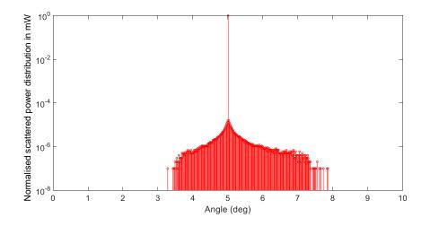
Figure 109 Example of single ray response of scattered ray, incident ray angle of 5°. A single incident ray is scattered into
