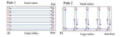
Figure 84 Stage moving paths for dynamic measurements. a): move horizontally first (bend position) and then move vertically (bend radius). b) move vertically first (bend radius) and then move horizontally (bend position).
