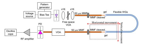
Figure 82 System setup for dynamic bending performance measurement. An 850 nm VCSEL was modulated by data via a bias tee. Then modulated laser light was coupled into flexible waveguides via a cleaved MMF. At the output side, the dashed sections were placed on a movable stage which can move horizontally and vertically. The corresponding power, bit error rate and eye diagrams were recorded.
