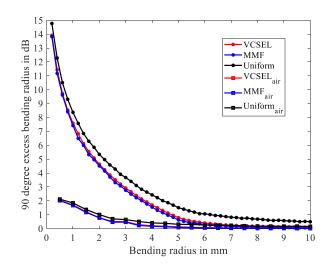
Figure 49 90° bending loss of normal waveguide structure and air-exposed structure under different launch conditions based on ZEMAX software.
