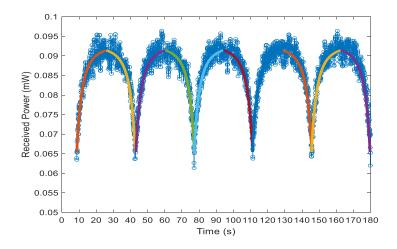
Figure 89 Vertical movement of dynamic measurement based on path 2, received power (markers) fitted using exponential curves (colour solid lines).
