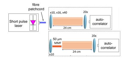
Figure 128 Investigation of mode excitation effects on the bandwidth performance of a flexible polymer waveguide. Short pulse laser was employed as input source and auto-correlator was used at output side to measure its AC pulse width. Flexible polymer waveguide was employed in the middle with different input launch conditions.
