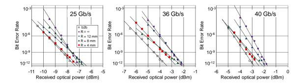
Figure 139 BER plots at 25 Gbps, 36 Gbps, and 40 Gbps for the b2b and waveguide links for the different radii applied to the 1 m spiral waveguide sample [170].
