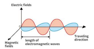
Figure 29 Scheme of electromagnetic wave, its electric field and magnetic field are oscillating and orthogonal with each other and also orthogonal with its propagation direction [109].
