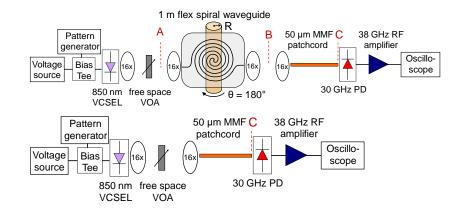
Figure 135 Experimental setup for the data transmission tests, back-to-back system was measured first as the reference results and then 1 m flexible spiral waveguide sample was employed into the system [170].
