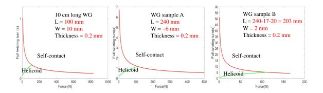
Figure 74 Phase diagrams of all three twisted flexible polymer waveguide samples. The maximum number of twist turns can be therefore obtained from the plots.
