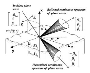
Figure 108 Geometrical arrangement to describe a local scattering event at a rough surface [148]. When ray hits the rough surface, both reflected scattered rays and transmitted scattered rays are generated.
