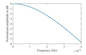
Figure 127 Optical spectrum of a 50 µm MMF input laser pulse based on Sech<sup>2</sup> curve fitting.
