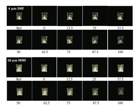
Figure 105 Near-field images of flexible polymer waveguide outputs as function of different squeezing distances under SMF and MMF inputs.
