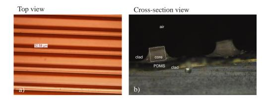
Figure 94 Top and cross-section views of bend-insensitive waveguide sample. a): top view, measured waveguide width is 52.58 µm. b): cross-section view, waveguide core is surrounded by a thin top cladding layer.
