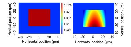
Figure 38 Refractive index profiles used in simulation for SI and GI waveguides. SI waveguide: with core RI value of 1.5255. GI waveguide: with maximum core RI value of 1.5255 and a parabolic-like RI pattern. Cladding values for both SI and GI waveguide are the same with the constant value of 1.5104.
