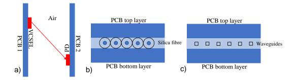
Figure 3 Three different methods for achieving optical interconnects, a) free -space connection, b) embedded fibre connection and c) polymer waveguide-based connection.
