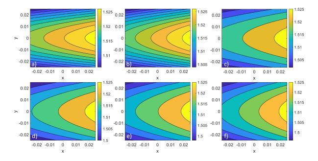
Figure 41 Different refractive index profiles of the waveguide core, RI changes in x direction linearly with a step value of 0.002. These six patterns are employed as waveguide RI profile during the simulation.
