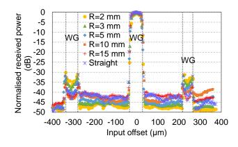
Figure 78 Normalised received power at the waveguide output as a function of the input position for different bending radii
