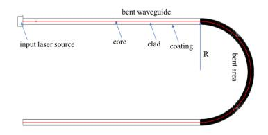
Figure 37 Simulation of bending loss performance system setup using ZEMAX software. The waveguide is formed of two straight sections and one bent section. Waveguide core cross-section is  $50 \times 50 \ \mu m^2$  surrounded by  $200 \times 200 \ \mu m^2$  cladding and a polyimide material layer is coated outside surface of cladding layer.
