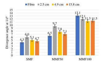
Figure 121 New far-field angles of waveguides in different lengths measured by ISO 11146-1 standard.
