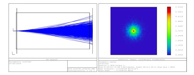
Figure 145 Simple demonstration of bulk scattering in polymer materials. A single input ray will generate hundreds of scattered rays after passing through a bulk material (bulk scattering).
