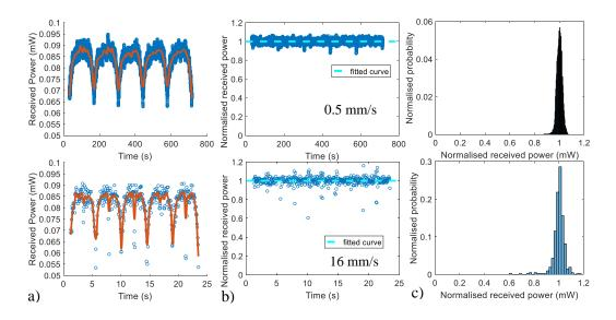
Figure 88 Vertical movement of dynamic bending measurement, a): received output power in mW, b): normalised output power based on mean value and c): corresponding histogram.
