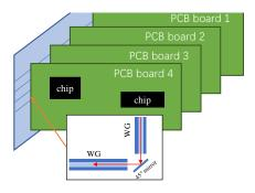
Figure 5 Schematic of board-to-board communications based on optical backplane topology. Four electronic PCBs are plugged into optical backplane and a 45° reflective mirror is employed to change the signal direction.
