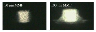
Figure 95 Near-field image of the bend-insensitive waveguide facet under 50 µm MMF and 100 µm MMF input launches.
