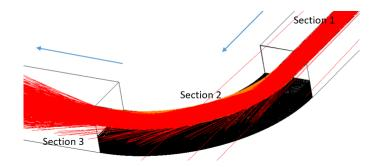
Figure 48 Waveguide structure in simulation of air-exposed waveguide model based on ZEMAX software. Section 1 and section 3 are straight waveguide sections and section 2 is bent waveguide section without top cladding. In section 2, waveguide core is directly exposed into the air.
