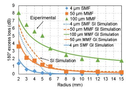
Figure 61 Excess bending loss for different bending radii under three launch conditions: experimental results (markers), simulation results with GI profiles (solid lines) and simulation results by employing SI profiles (dash lines).
