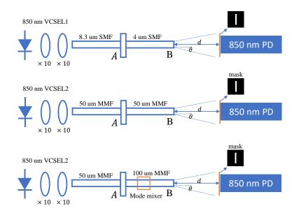
Figure 52 System setup for measuring far-field distribution of fibres. Laser light was coupled into the fibre first via a pair of  $\times 10$  lenses. A mask with a 1 mm wide slot in the centre is placed in front of the broad-area photodetector (PD).
