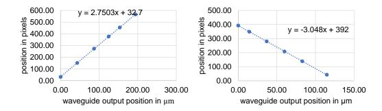
Figure 119 Relationship between distance in pixel values and µm values. Slop values indicate how many pixels can represent
