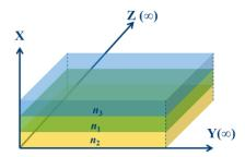
Figure 24 Parallel planar waveguide model, three layers with infinite width (Y) and length (Z).
