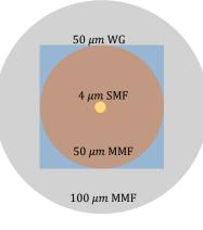
Figure 57 Mathematic illustration of the geometry mismatch between the waveguide and different fibre inputs.
