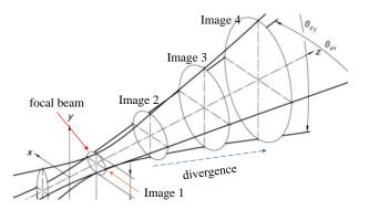
Figure 116 Schematic of a divergent beam [153]. Bean width is the smallest at focal plane.
