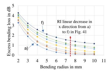
Figure 42 Simulated bending loss performance of waveguides for different RI profiles under 50 µm MMF, RI changes in a linear decay in the x-direction. 'pattern a' results in the best loss performance while 'pattern f' results in the worst.
