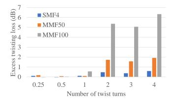
Figure 70 Average excess twisting loss for the 10 cm flexible polymer waveguide sample as a function of twisting numbers. When number of twist turns is bigger than 1, twisting nodes are generated, which results in bigger loss. Three different input launches are employed.
