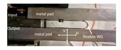
Figure 83 Image of flexible polymer waveguide confined by two metal pads in dynamic system setup. Pads employed here to confine the shape of bent waveguide sample.
