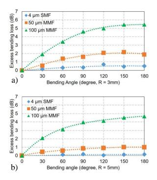
Figure 64 Excess bending loss as a function of bending angle for (a) 3 mm and (b) 5 mm radius for the three launch
