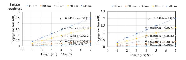
Figure 107 Simulation of propagation losses as a function of waveguide length due to different surface roughness. Slope values are the propagation losses and inception values are coupling losses (almost 0).
