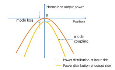
Figure 102 Schematic diagram of mode loss and mode coupling schemes. Mode loss refers to the total power loss while mode coupling refers to the coupling process between different modes. Power reduction for a specific mode is consist of mode loss and mode coupling.
