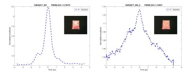
Figure 141 AC traces of waveguide output pulses under two different launch conditions. Restricted launch condition results in a better and clearer curve while over-filled launch generates a bad curve and poor fitting.
