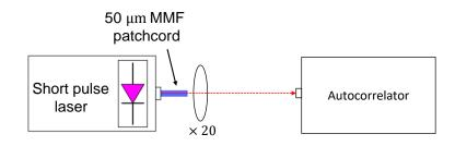
Figure 125 Back-to-back system setup of the ultra-short pulse measurement using 50 µm MMF as the input launch. Autocorrelator measures the pulse that directly from short pulse laser.
