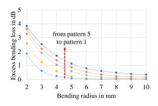
Figure 44 Simulated bending loss performance of waveguides for different RI profiles under 50 µm MMF, with RI changes in the y-direction (parabolic shape is changed).
