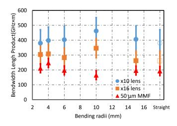
Figure 132 Bandwidth length product (BLP) of the flexible polymer waveguide sample under flexure. Several bending radii were employed and three different launch conditions were used.
