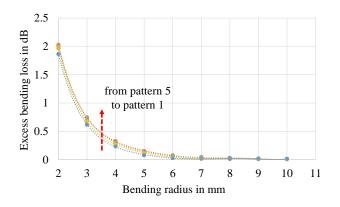
Figure 45 Simulated bending loss performance of waveguides for different RI profiles under SMF launch.
