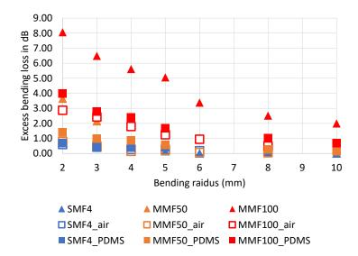
Figure 97 Excess bending losses of the bend-insensitive waveguide for different bending directions in comparison with a
