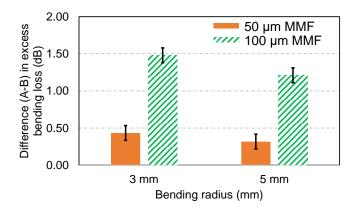
Figure 67 Difference in excess bending loss between directions A and B when the sample is bent 180° with a 3- and 5-mm radius, respectively. Positive values mean that the bending loss in A configuration is higher than the bending loss in B configuration.
