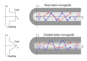
Figure 36 Refractive index profile and path trajectories of step-index and graded-index waveguides. Dispersion generated in GI waveguide is smaller than SI waveguide due to the faster transmission speed of the rays with bigger incident angle [132].
