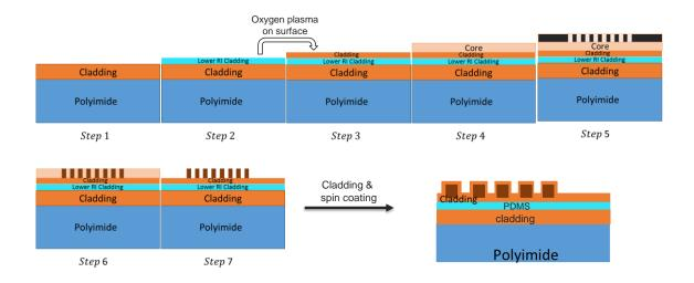
Figure 93 Fabrication steps of flexible polymer waveguides for the new proposed bend-insensitive structure.
