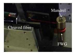
Figure 59 Image of the bent waveguide sample illuminated with red light.
