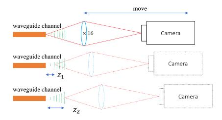
Figure 117 System setup for measuring far-field profile based on ISO 11146-1 standard. Un-focused near-field images at different positions together with focused image at focal plane were recorded.
