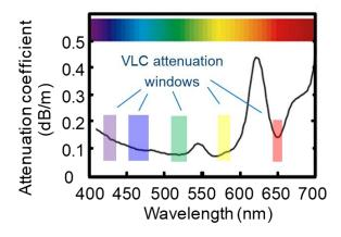
Figure 8 Loss spectrum of PMMA material, several attenuation windows are indicated in visible light range and the unit of
