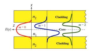
Figure 27 Electric field patterns of first three modes (m = 0, 1, 2) in planar waveguide. Exponential decay profiles are seen from cladding regions [108].
