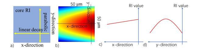
Figure 40 a) Schematic structure of graded-index profile distribution. b) generated graded-index RI profile for waveguide core in simulation. c) linear decrease of RI value in x-direction, cut from horizontal dash line in b. d) parabolic shape of RI value in y-direction, cut from vertical dash line in b.
