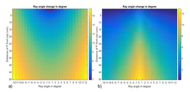
Figure 47 a) Ray angle generated in the bent waveguide section as a function of ray angle and ray position in straight waveguide section. b) ray angle difference of the same ray measured in straight waveguide and in bent waveguide as a function of ray position and ray angle.
