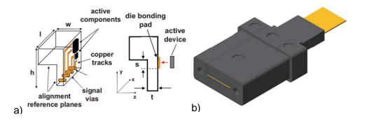
Figure 23 Examples of end-butt coupling elements a) L-shape connector and b) Pluggable polymer MT connector [99, 100].
