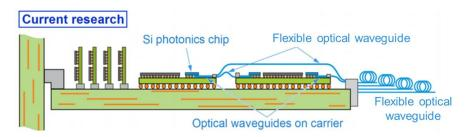
Figure 6 Optical polymer waveguides connecting chips assembled on carriers. Flexible optical waveguides are employed to make chip-to-chip and board-to-board communications as suggested in figure [51].
