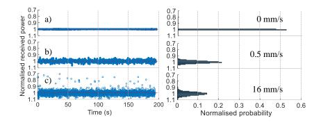
Figure 86 Normalised received power at the waveguide output over time and the corresponding histogram when (a) there is no movement, (b) a slow (0.5 mm/sec) and (c) a fast (16 mm/sec) dynamic movement applied.
