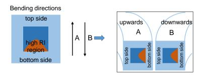
Figure 66 Schematic illustration of the two out-of-plane bending directions. Due to the asymmetric RI profile, different bending directions will generate different configurations (A and B).
