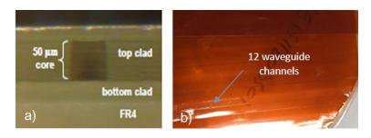
Figure 11 Siloxane polymer waveguide samples, a) cross-section view: squared-shape polymer waveguide core in the middle of cladding with FR4 substrate and b) top view: 12 parallel waveguides are deposited on polyimide substrate.
