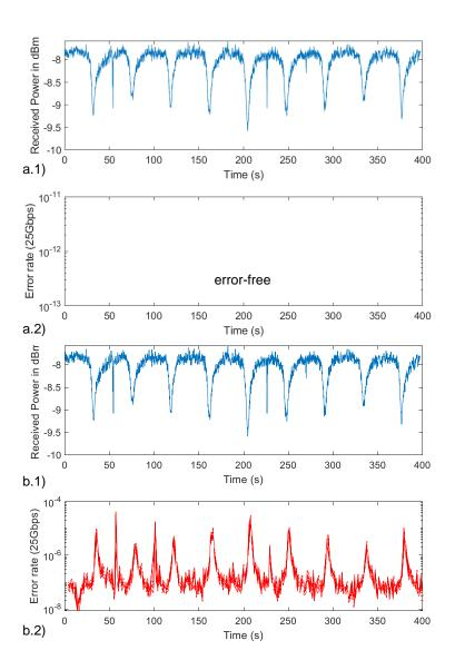
Figure 91 Bit error rate performance as a function of received power under dynamic bending measurement for 25 Gbps transmission, a) received power was set to be -0.5 dBm and b) received power was set to be -8 dBm.
