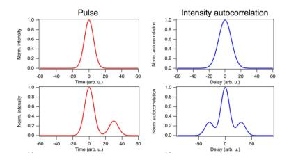
Figure 140 Laser pulses with post-sub peaks and their resultant AC traces [171].
