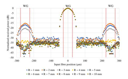
Figure 76 Simulation of the normalised received power at the waveguide output as a function of the input source position for different bending radii for the 50 µm MMF input. Waveguide positions are indicated by red dash lines.
