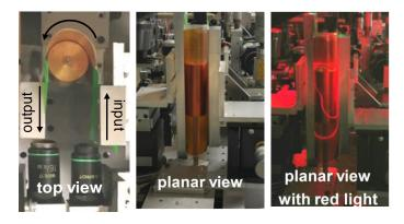
Figure 136 Images of the sample wrapping around the mandrel of 12 mm radius and illuminated with red light.
