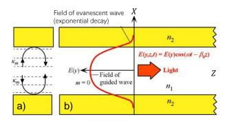
Figure 26 a): Upward and downward travelling waves have equal but opposite wave vector, which could form standing waves between two boundaries. b): electric field of lowest (m=0) mode inside planar waveguide [108].
