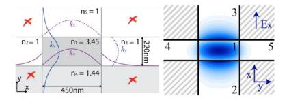
Figure 32 Sketch of fundamental mode profile of a rectangular waveguide and its TE-like mode simulation [114]
