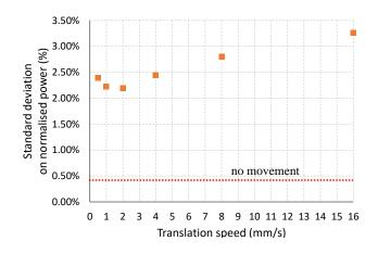
Figure 90 Obtained standard deviation values as a percentage of the mean value of the received power for different
