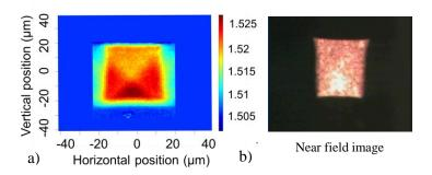
Figure 51 a) Measured refractive index profile of the real waveguide sample and b) its near-field image of the waveguide output facet (illuminated by 850 nm laser light)
