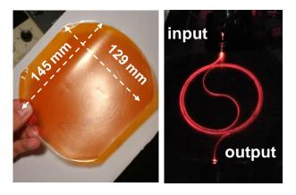
Figure 134 Image of flexible waveguide sample with size noted and a 1 m long spiral waveguide illuminated with red light. Waveguide sample was provided by Dow Corning.
