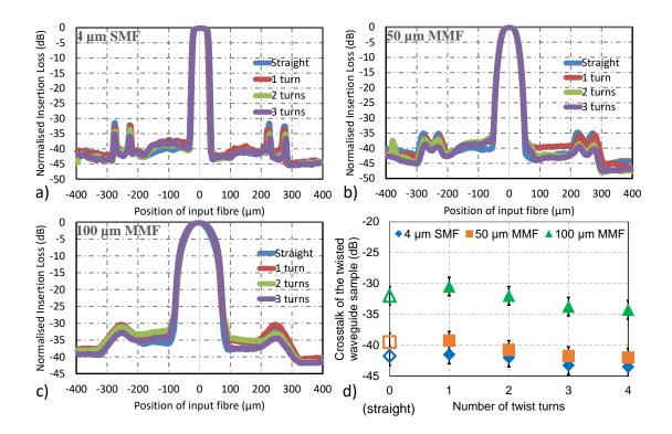
Figure 81 Normalised received power at the waveguide output as a function of the input position for different bending radii a) SMF; b) 50 μm MMF input; and c) 100 μm MMF input. d) Summary of the crosstalk of a twisted sample for different numbers of full twisting turns and the different launch conditions.
