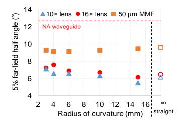
Figure 133 5% far-field half angle of the waveguide output laser beam. Numerical aperture (NA) of the waveguide is indicated by red dash line. All the launches employed during the experiment were under-filled (below red dash line). The 5% FFAs of straight flexible polymer waveguide are also measured as the reference.
