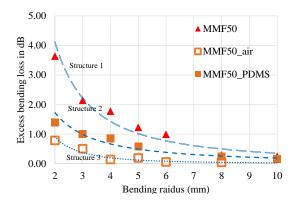
Figure 96 Excess bending losses of bend-insensitive waveguide facing different directions in comparison with traditional waveguide. Loss performance of tradition waveguide is indicated by triangle markers. MMF50\_air (unfilled rectangular markers) means that thin top cladding layer facing outside when bending the waveguide while MMF50\_PDMS (filled rectangular markers) means that thin top cladding layer facing layer fac
