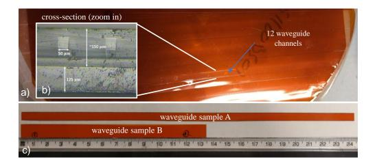
Figure 50 a) Flexible polymer waveguide samples used in this work, provided by Dow Corning company. b) cross-section view of the flexible polymer waveguides, facet is not polished. c) two flexible polymer waveguide samples with different
