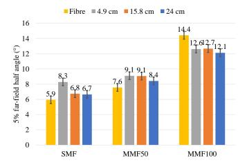
Figure 115 5% FFAs of straight flexible polymer waveguide samples for different lengths under different launch conditions.
