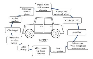
Figure 7 Generic architecture of Media Oriented Systems Transport (MOST) data bus system. Each unit is connected via POF link based on ring topology.
