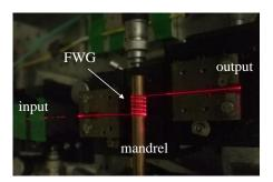
Figure 99 Experimental setup for the small bends effect on a flexible polymer waveguide which is illuminated with red laser light. Here, waveguide sample was bent by 5 turns.
