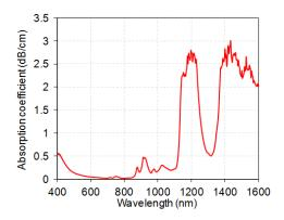
Figure 10 Measured propagation loss of Dow Corning siloxane material within the wavelength range from 400 nm to 1600 nm. Lowest loss value at around 850 nm wavelength window which is less than 0.05 dB/cm [36].
