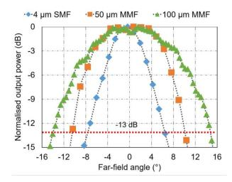
Figure 53 Far-field intensity profiles of three different launch conditions. Intersection points between intensity profiles and the horizontal red line (-13 dB) are corresponding to the 5% far-field angles. 4 µm SMF is used to simulate restricted launch condition, 50 µm MMF is used to simulate most common launch condition and 100 µm MMF is employed to simulate overfilled launch condition.
