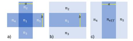
Figure 31 a) Configuration of the rectangular dielectric waveguide, b) equivalent confinement of a 1D guide in the y direction and c) equivalent 1D guide with confinement in the x direction
