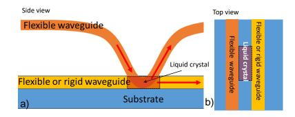
Figure 144 a): side view of new coupler design by introducing liquid crystal in intersection region. b): top view of the new coupler design, curved waveguide is not placed at the same plane as straight waveguide.
