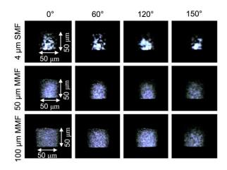
Figure 65 Near-field images of the waveguide output for different bending angles for a 3-mm bending radius under three launch conditions. 0° means waveguide sample is in straight condition.
