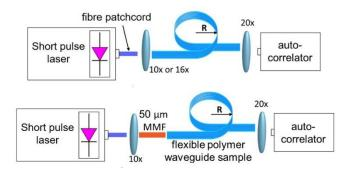
Figure 131 Experimental setup for bandwidth studies using a lens launch and a 50  $\mu$ m MMF input.
