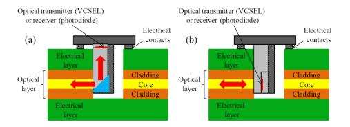
Figure 16 Two essential coupling schemes: a) out-of-plane coupling and b) in-plane coupling. In out-of-plane coupling scheme, the active components are located at the different layer from polymer waveguide while in in-plane coupling scheme, the active components are placed at the same layer as polymer waveguide [95].
