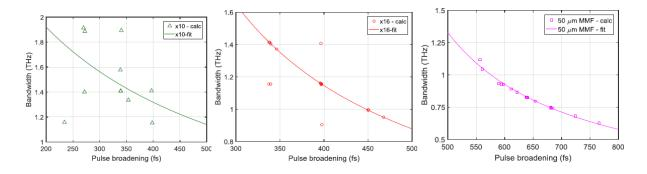
Figure 142 Bandwidth values as a function of pulse broadening.
