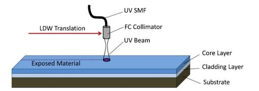
Figure 14 Schematic of laser direct writing process for the fabrication of polymer waveguides. Core material is photo-sensitive and being polymerised by focused UV light. The waveguide core size is controlled by the scanning speed and UV beam size. Both single mode waveguide and multi-mode waveguide can be made using laser direct writing method [89].
