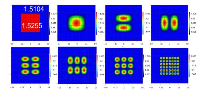
Figure 33 Simulation of optical modes for  $50 \times 50 \ \mu m^2$  waveguides under 850 nm wavelength based on OptiBPM software. Refractive index values for core and cladding are set to be 1.5255 and 1.5104, respectively, which are close to the values measured from the real waveguide samples.
