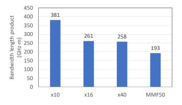
Figure 130 Bandwidth length product (BLP) of a straight polymer waveguide under different launch conditions.
