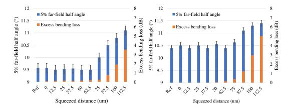
Figure 104 Obtained 5% FFAs and excess losses for the 24 cm long waveguide as a function of the reduction in separation distance between the indentation teeth under 4 µm SMF (left) and 50 µm MMF inputs (right)
