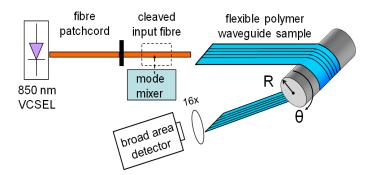
Figure 63 Experimental setup for the bending angle effect. Flexible polymer waveguide sample was bent on a mandrel with different bending angles from 0° to 180°.
