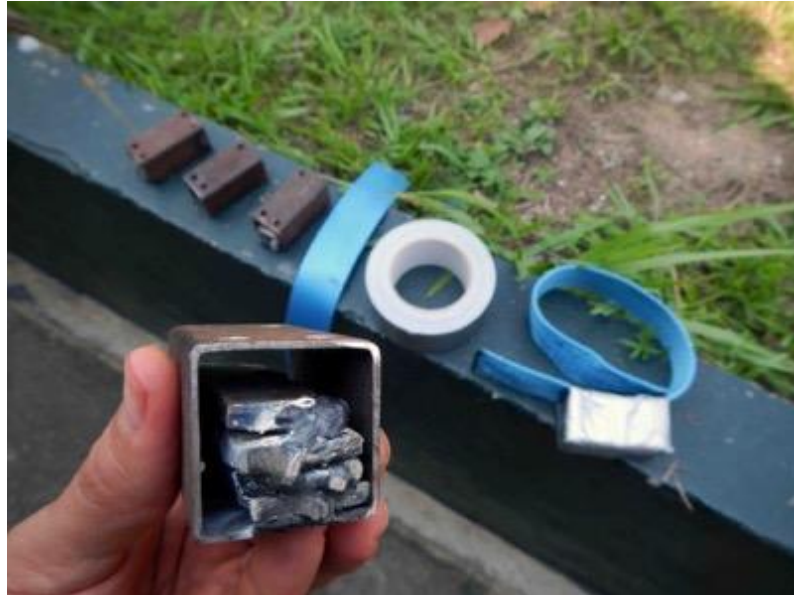
Figure 2.19 Unassembled practice collar with internal weights in hand and finished collar wrapped in duct tape resting on retaining wall
