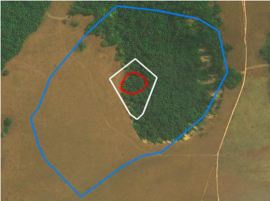
Figure 4.3 Kernel Utilisation Distribution Density of GPS collars in the stationary collar test. The blue polygon was created using 3D points collected at 0.5 m. The white polygon was created using the 3D points collected at 21 m and the red polygon was created using 3D points collected at 29 m.
