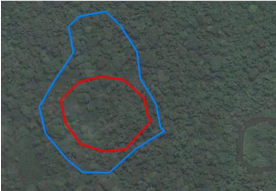
Figure 4.4 Kernel Utilisation Distribution Density of the height in the canopy test. The blue polygon was created using 3D points collected at 0.5 m. The red polygon was created using 3D points collected at 18.8m.
