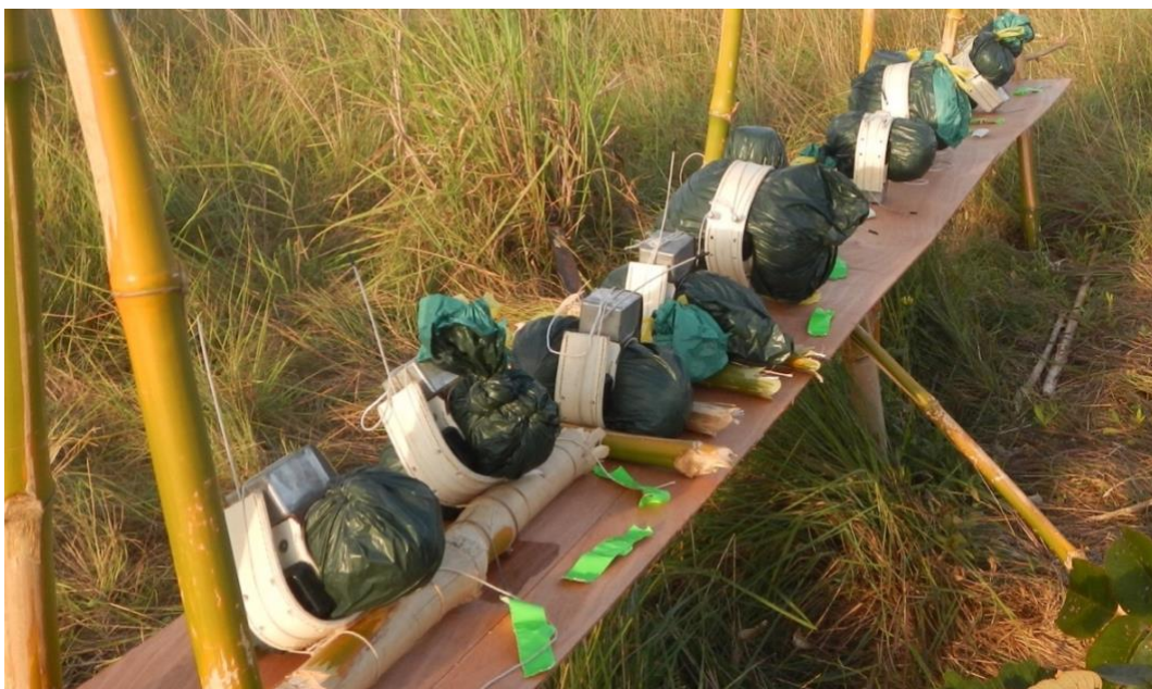
Figure 3.2 Collars fitted to simulated animals, placed on platform in open savanna. The collars were oriented at 0^\circ , 45^\circ , 90^\circ , 135^\circ and 180^\circ to test for an effect caused by collar orientation.
