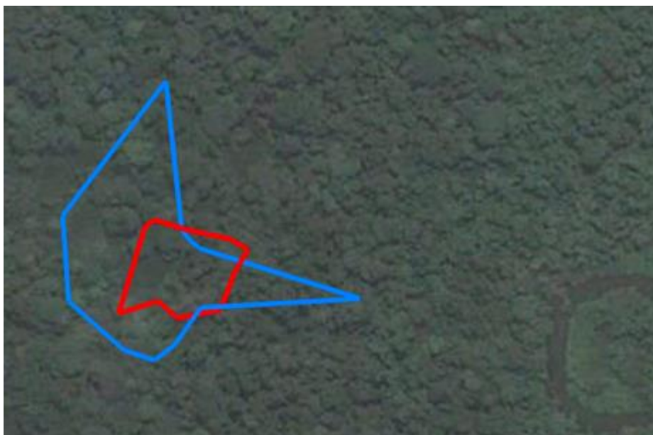
Figure 4.5 Local Convex Hull (95%, Neighbours: 30) density of GPS collars in height in the canopy test. The blue polygon was created using 3D points collected at 0.5 m. The red polygon was created using 3D points collected at 18.8 m.
