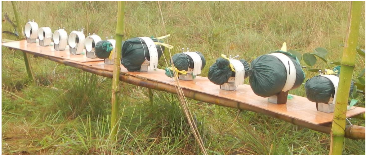
Figure 3.1 Empty collars and collars fitted to simulated animals placed upright on a platform in open savanna.
