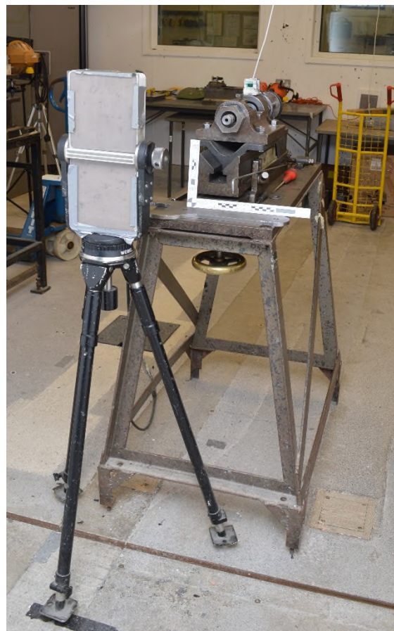
Figure 4: Proof housing with 127 mm barrel and Weibel Doppler radar to the left facing down the range
