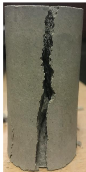
c. Cone-split collapse after 72 h of curing at 40°C, LP=21%
