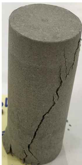
b. Cone-shear collapse At 24 h of curing at 40°C, LP=25%
