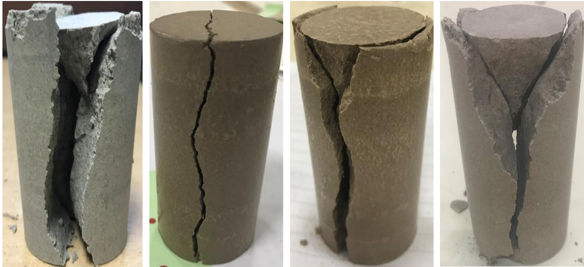
a. M1 Lime treated bentonite LP = 17% and T = 40°C b. M2 Lime treated ball clay LP = 13% and T = 20°C c. M3 Lime treated 1:3 bentonite – ball clay LP = 9% and T = 40°C d. M4 Lime treated 1:1 bentonite – ball clay LP = 13% and T = 40°C
