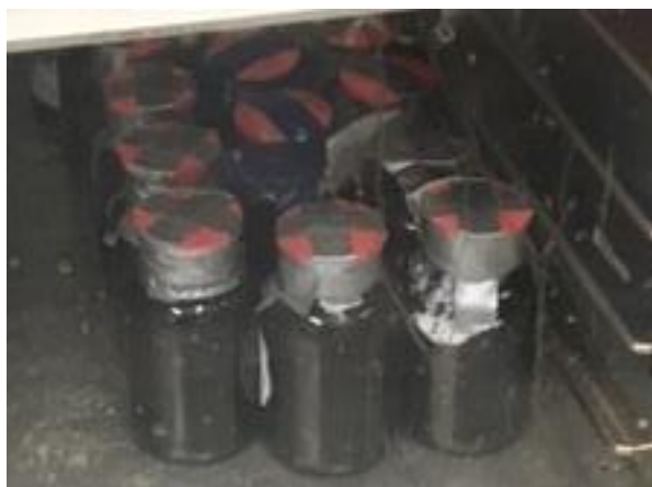
Figure 8-3 Anaerobic biodegradation test sample bottles
