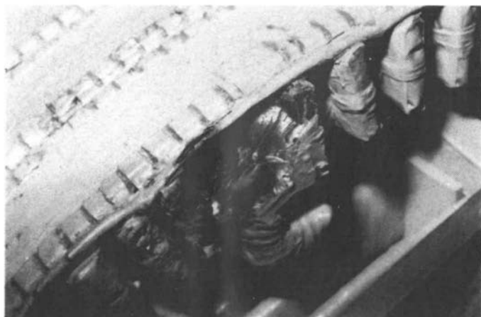
Fig. 10 Damage to the wound rotor of a 4.8 MW induction motor detected by gas monitoring
