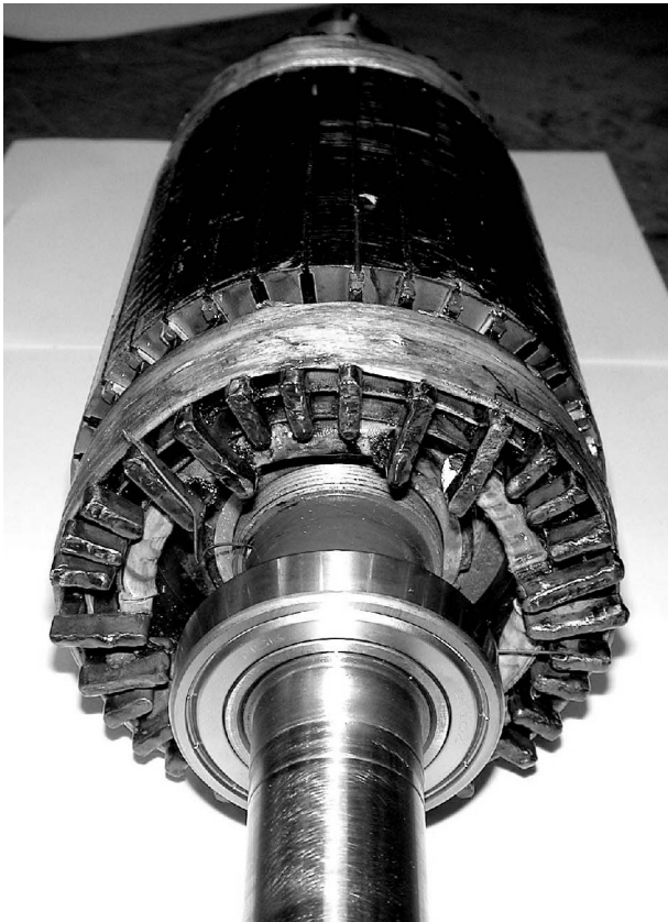
Fig. 3 Rotor 3: Prototype new double layer design
