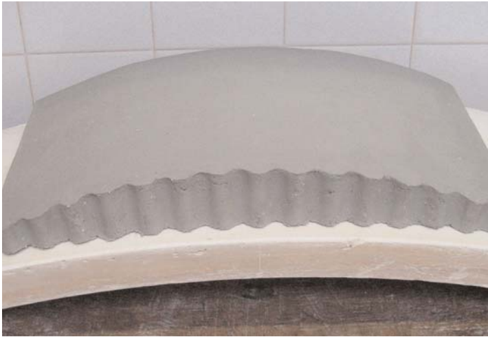
Pressed and shaped corrugated edged standing form.
