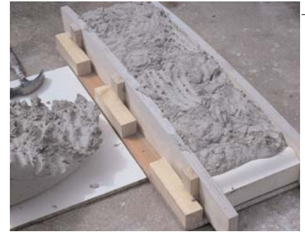
Filling a long boat mould with stained, aggregate bearing porcelain.
