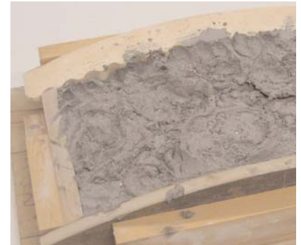
Pressing and shaping of corrugated edged standing form – adjustable wood and plaster mould, with corrugated insert.
