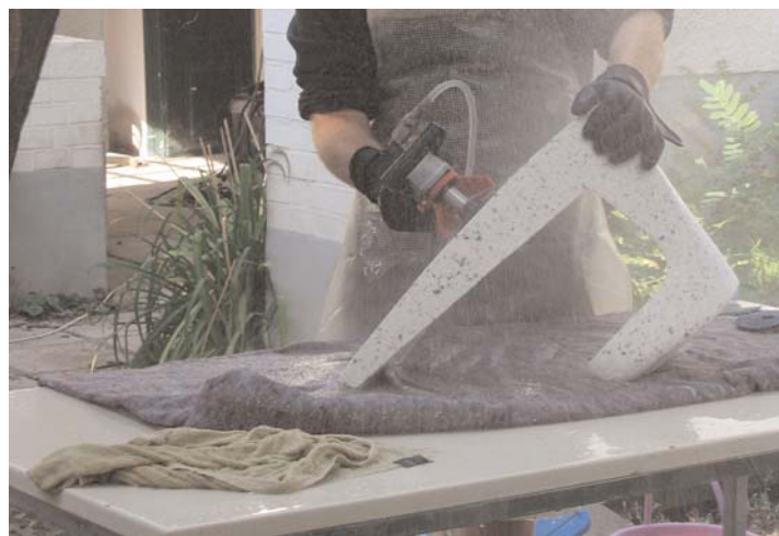
Grinding fired form at International Ceramics Studio, Kecskemét, Hungary.
