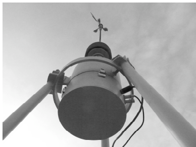
Fig. 3. The weatherproof camera housing and weather station installed at the top of the Monument ( Photo © Chris Meigh-Andrews)
