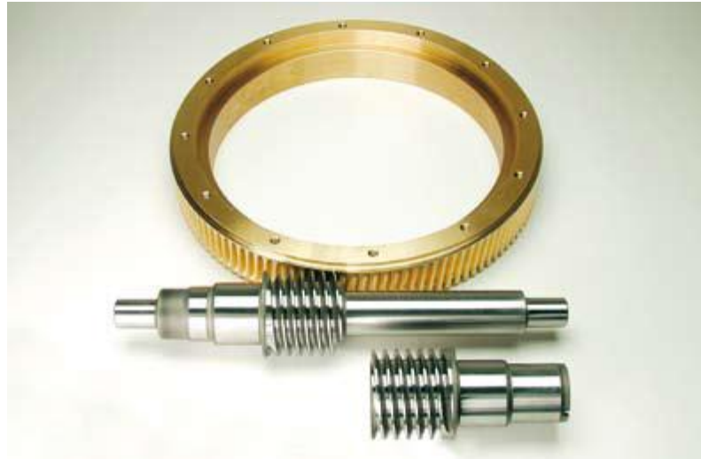
Figure 67- OTT anti backlash worm and wheel (zahnrad-ott, 2012)
