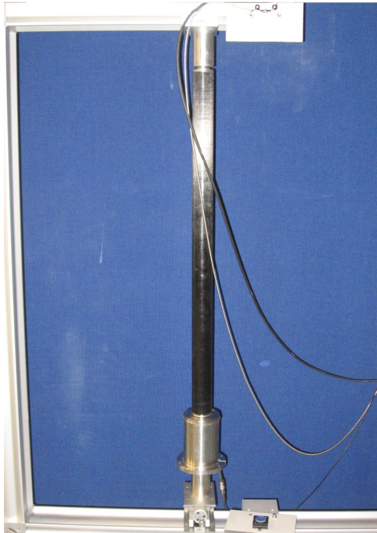
Figure 94- Actuator leg under test
