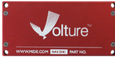
Figure 41 – Volture piezo energy harvester (Mide, 2012)
