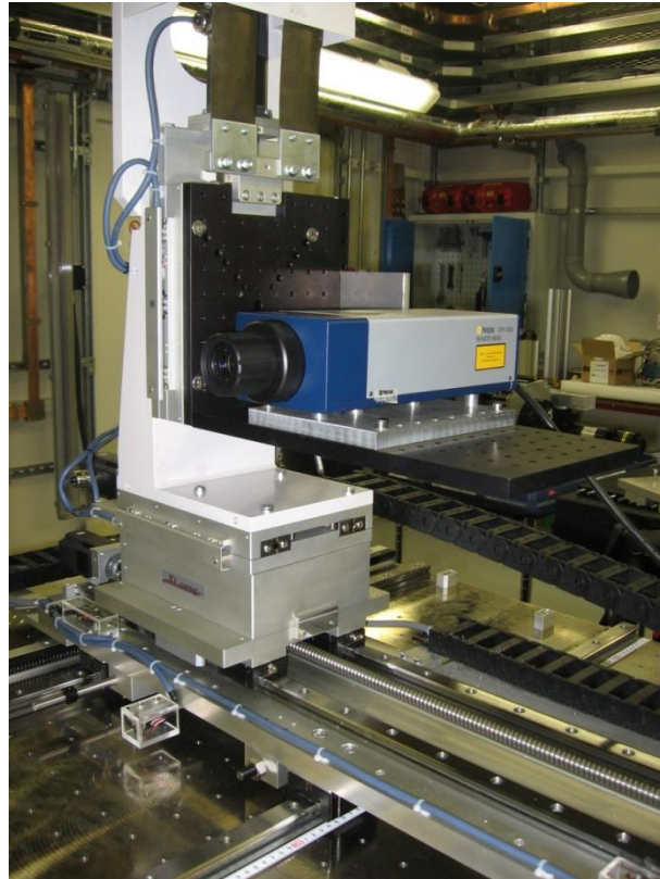
Figure 105 – Vibrometer mounted on detector stage
