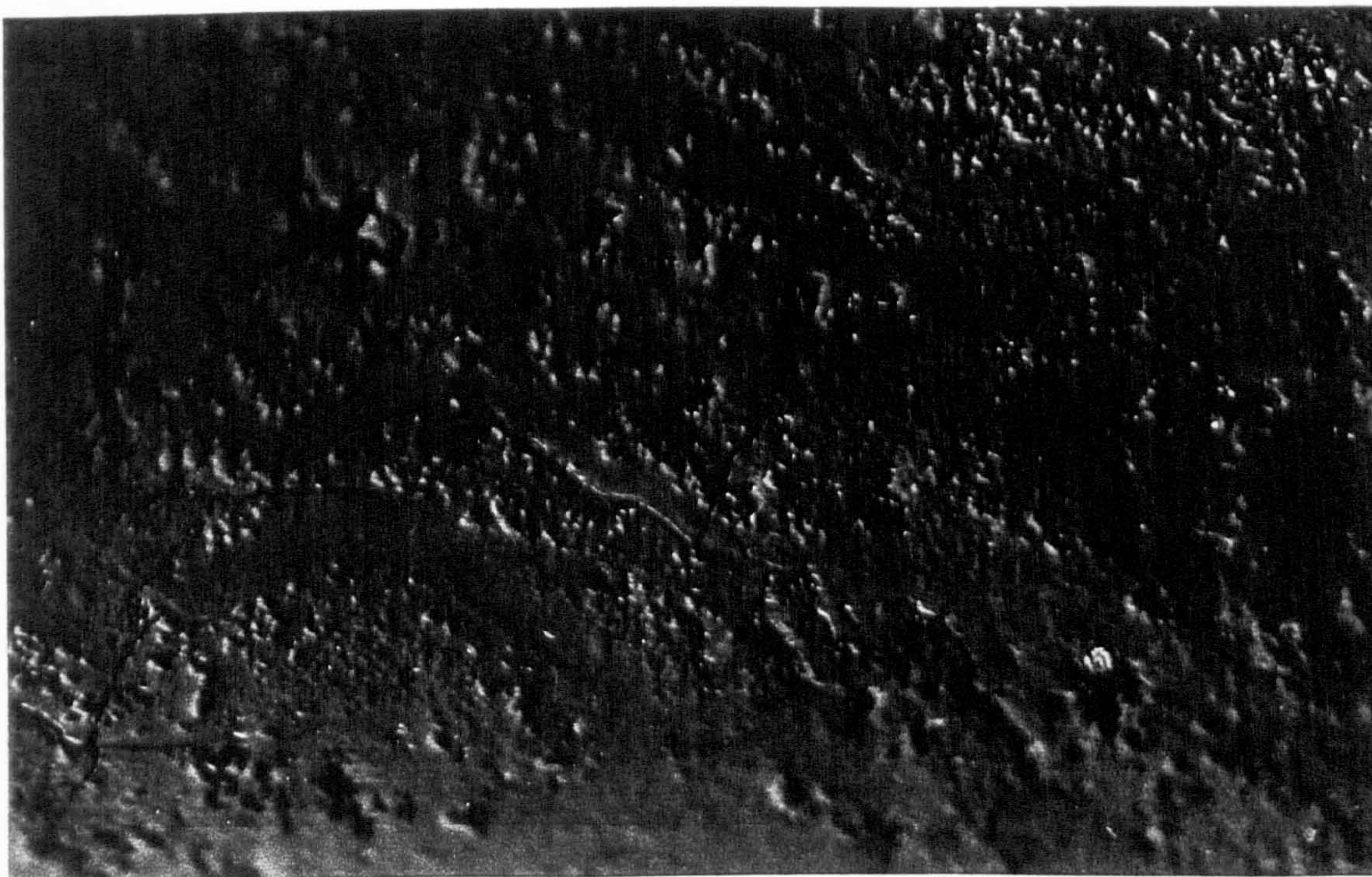
Fig. 4.204 - Sectioned pin - unetched DIC x 1000
