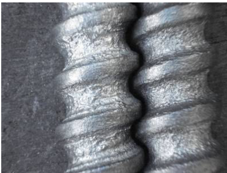
Figure (6-1): Shows the self wiping and intermeshing action of the screws.
