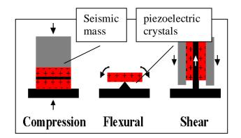
Fig.2.6.3e Types of configurations.
