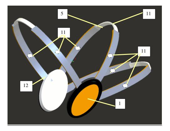
Fig. 6.1e Watch electrode-antennas are separated(proEngineer)
