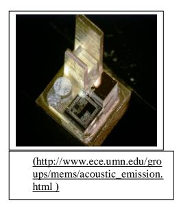
Fig.2.7.6 Integrated AE sensor (mm range).
