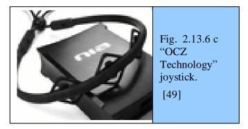
Next is the OCZ company joystick, built by "OCZ Technology" (California - Mar/2008). Similar to the Belgian thermal energy EEG (Fig. 2.13.6d), this product is also made out of 3 dry electrodes for signal identification. The above photo clearly shows the 3 diamond shaped parts of the black bow which goes over the head of the
