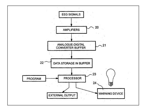
Fig. 2.11.4 An EEG processor with a user-warning Algorithm. [33]
