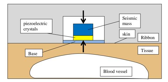
Fig . 5.5.3c Force piezoelectric sensor. [59]
