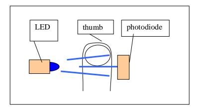
Fig. 2.8.2 Direct infrared probing method.
