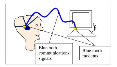
Fig. 5.6.4d Bluetooth communications. (rejected design solution).
