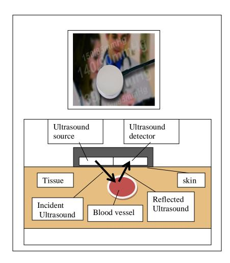
Fig.2.7.1b Diagram and photo of Ultrasonic blood pressure sensor. [11]
