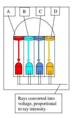
Fig.5.5.3f One photodiode containing 4 smaller selective photodiodes. [65], [66]
