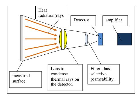
Fig. 5.5.3d MEMS Infrared Thermometer Diagram.[60],[61],[62]
