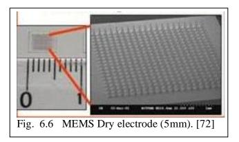
These electrodes will save a lot of space because they have mm dimension range, unlike other usual electrodes which are much larger in size. The electrodes are wireless sending physiological signals to the watch processor without the use of wiring. These miniaturised electrodes has the ability to ignore or eliminate extraneous body movements and signals and detect only the desired scope of signals (physiological signals).
