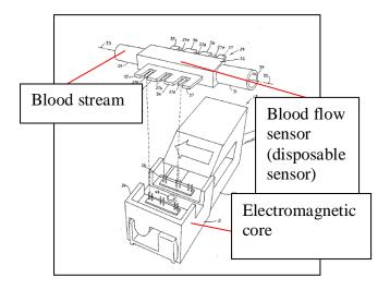
Fig. 2.9a Disposable and invasive electromagnetic BP sensor. [23]
