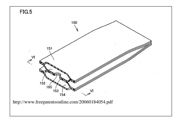
Fig 4.1 (c) Inflatable device structure, 8/2006
