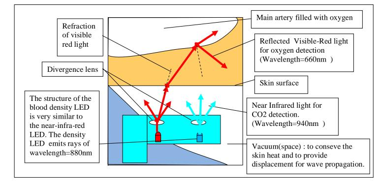
Fig. 5.5.3e Oxygen/CO2 sensor (width = 3mm). [64]
