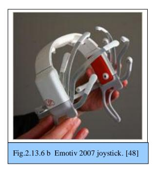
This is Emotiv's second brainwave control headset (2007) with 14 electrodes (Fig. 2.13.6b). The processor is separated from the helmet (wireless). The product is also used for video games control, but it is fairly smaller in size than the old version. The lower curves shown on the above photo clips to the ears to give the product a firm hold on the head.
