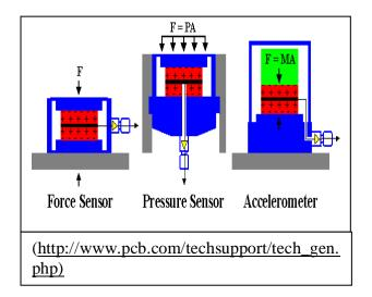
Fig.2.6.3d Types of piezoelectric sensors. [9]
