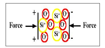
Fig. 2.6.3c Rearrangement of charged particles.
