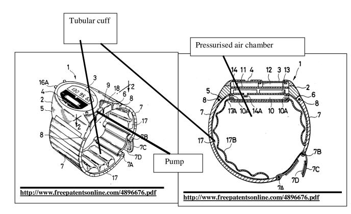
Fig. 4.1 (b) Small Blood-Pressure Watches with a tubular cuff (automatic inflation)
