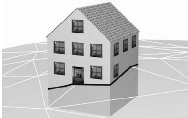
Figure 3. CityGML's 'TerrainIntersectionCurve' (shown in black), a 3D polyline representing where the building meets the terrain. Source: Groger et al. (2006).
