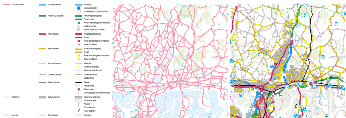
Figure 7. 'The Map is the Legend'. Digital prototype with legend items arranged hierarchically (left), styled hierarchically (centre) and styled according to current Digimap convention (right).
