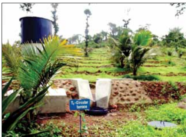
Installation of gauging stations for measurement of run-off and soil loss in coconut
