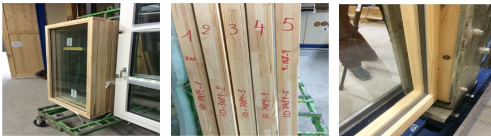
Figure 3. Three vacuum glasses (1,2,3) and two conventional double-glazed samples (4,5) and their installation into the clamping frame of the pendulum setup
