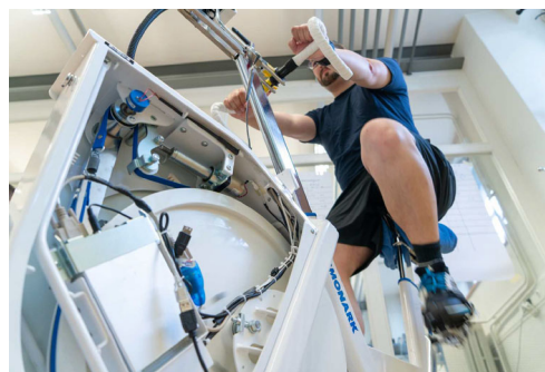
Fig. 3 Computer-controlled cycle ergometer (Monark LC7)
