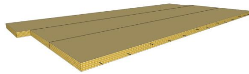
Figure 12. Post-tensioned working platform
