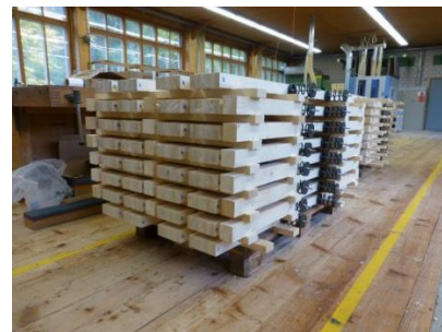
Figure 8. Long-term bending tests on butt joint bonded CLT-beams.
